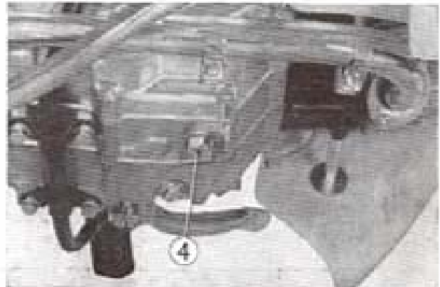
① Filler cap dipstick ② Lower level mark ③ Upper level mark ④ Oil drain plug
