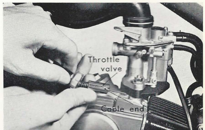
Figure 4-4. Disconnect cable from throttle valve
