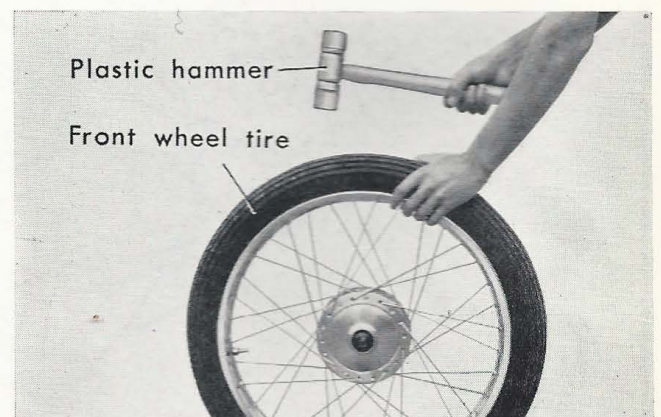
Figure 4-23. Tap the tire all around with a hammer
