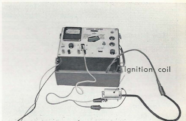
Figure 5-11. Testing ignition coil
