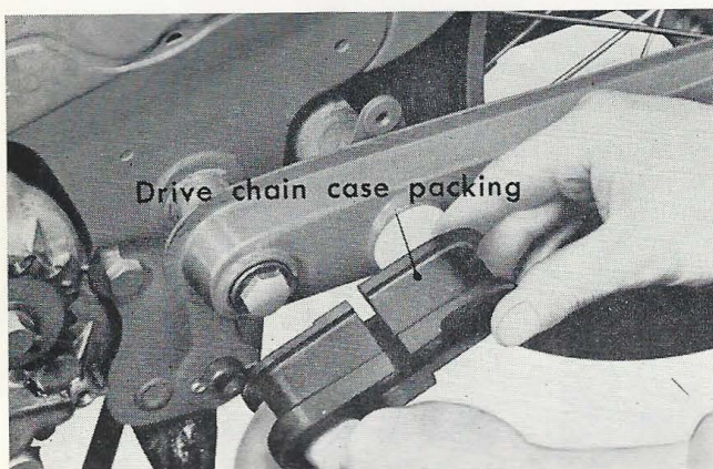
Figure 4-43. Installing chain case packing
