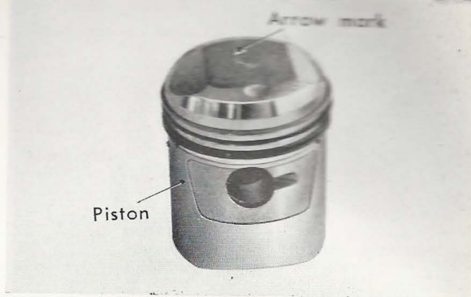
Figure 3-55. Arrow marking on piston head
