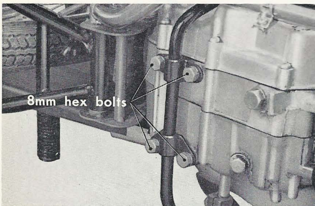
Figure 4-37. Installing step bar
