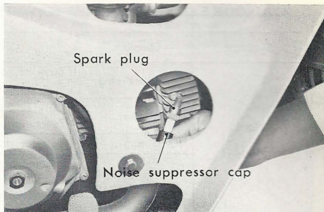
Figure 5-10. Testing spark plug firing
