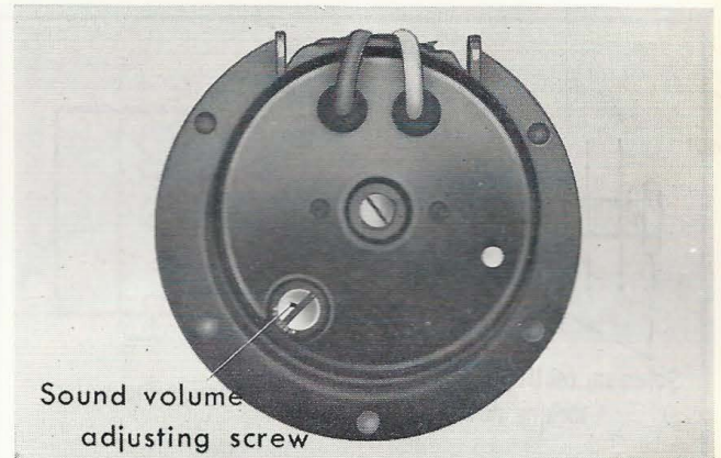
Figure 5-35. Adjusting the horn
