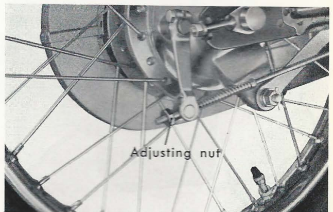
Figure 6-38. Adjusting rear brake
