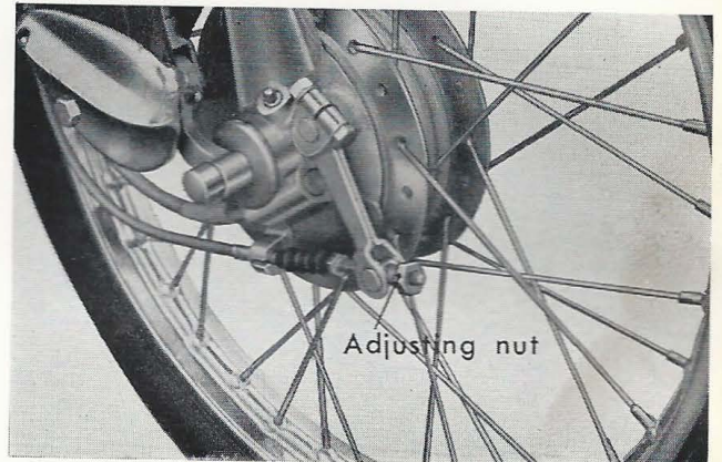
Figure 6-36. Adjusting front brake lever
