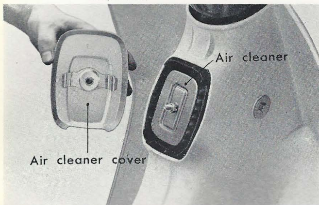
Figure 4-48. Removing air cleaner (C50, C50M, C65, C65M)
