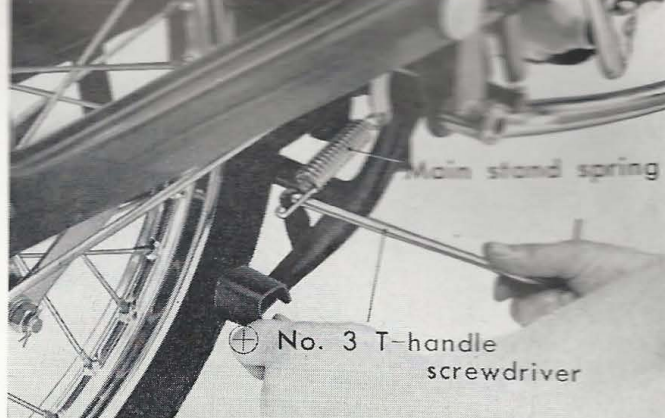
Figure 4-38. Installing stand spring
