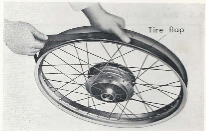
Figure 4-22. Installing tire flap
