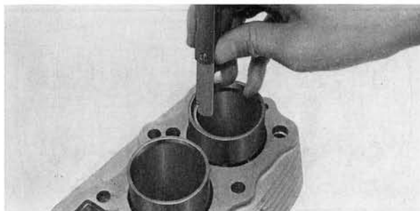
Fig. 3-16 Checking piston ring end gap
