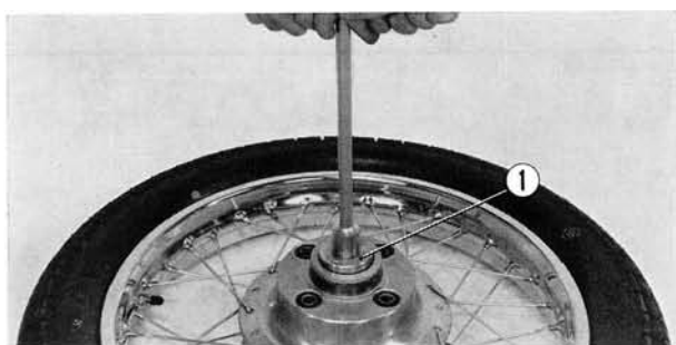
Fig. 4-29 ① Bearing retainer wrench
