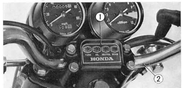
Fig. 4-36 ① Upper handle holder ② Steering handlebar
