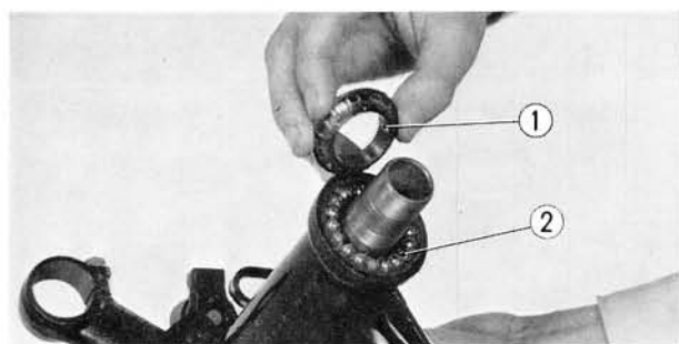
Fig. 4-45 ① Top cone race ② #8 steel balls
