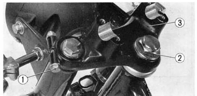
Fig. 4-43 ① Front fork bolts ② Steering stem nut ③ Fork top bridge
