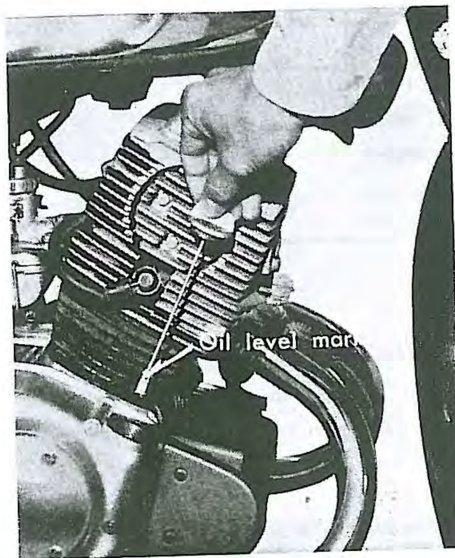
Fig. IV-19. Checking oil level
