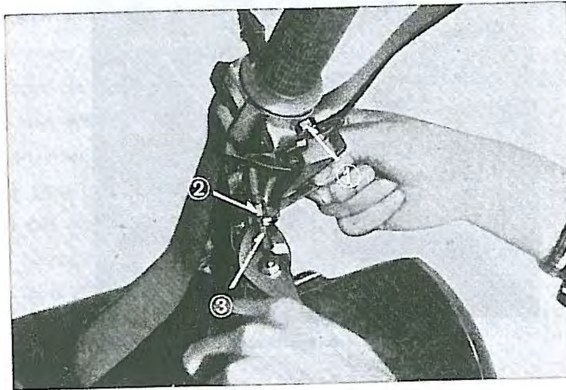
Fig. IV-16. Throttle adjustment (C92)
