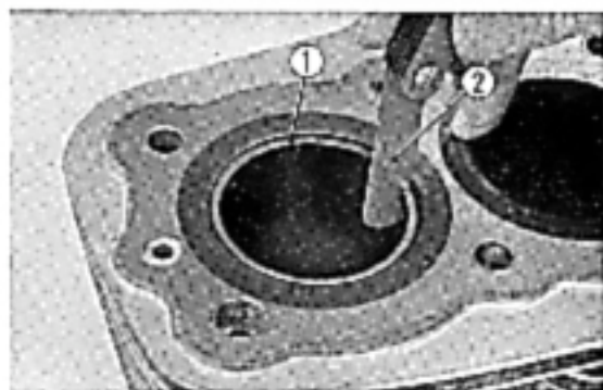
Fig. 72 ① Piston ring ② Feeler gauge
